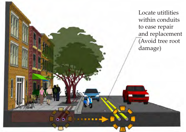
Figure 1: Move underground utilities under bike lanes
