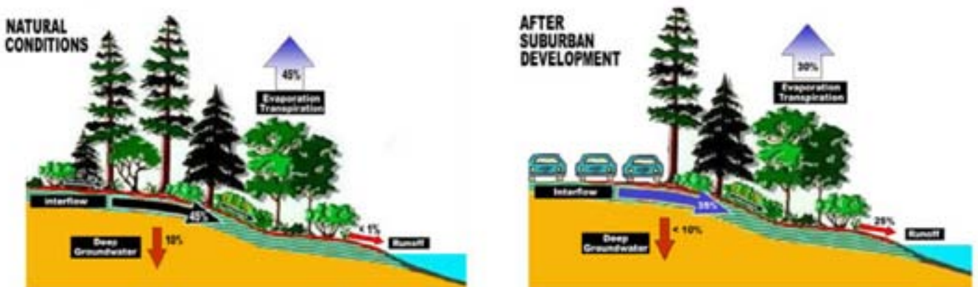
Figure 10: Water balance before and after suburban development
